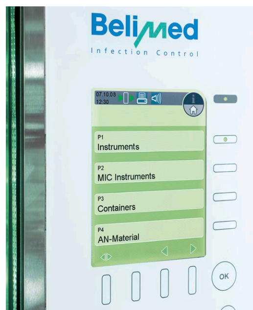
Uniform CP-TOP operating panel, behind glass, with function buttons in touch screen technology
