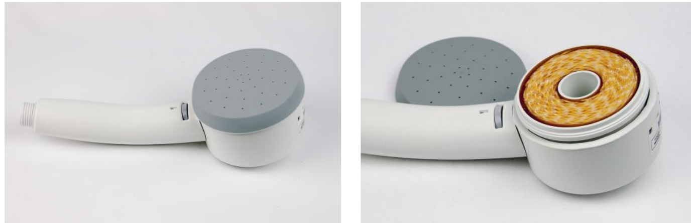
Figure 2: Evaluation of Shower Filter for defects and discolourations
