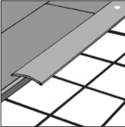
Figure 20 Threshold strip
