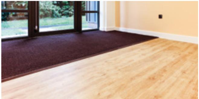
**NOTE** To maintain the effectiveness of dirt barrier systems, they must be cleaned regularly, otherwise they can actually increase the soil intake by creating a ‘soil reservoir’ at the entrance to the building.
