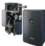
"Regumaq X-45" Fresh water station with intuitive touch display for the setting of different functions such as circulation, return temperature layering or heat demand. The operating element made of safety glass is integrated in the front insulation shell and is connected to the controller box without plug via magnetic contacts.
