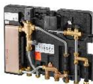
"Regudis W" Dwelling station Dwelling station with plate heat exchanger for heat transmission from a central heat supply to the sanitary and heating installation of a dwelling
