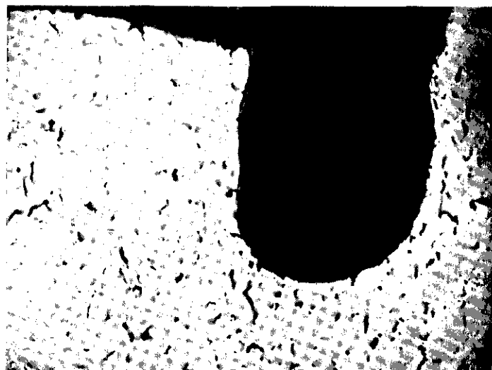
Fig. 7. Photomicrograph of a cross-section taken from the tube showing one of the deep pits, decarburisation of the steel and numerous micro-cracks.
