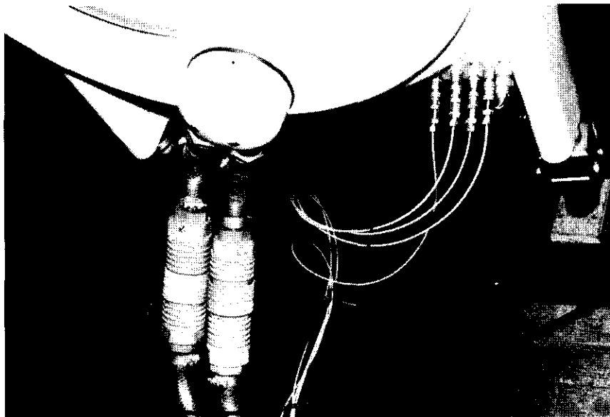
Figure 3: Extract hose connections with quick-release device.
